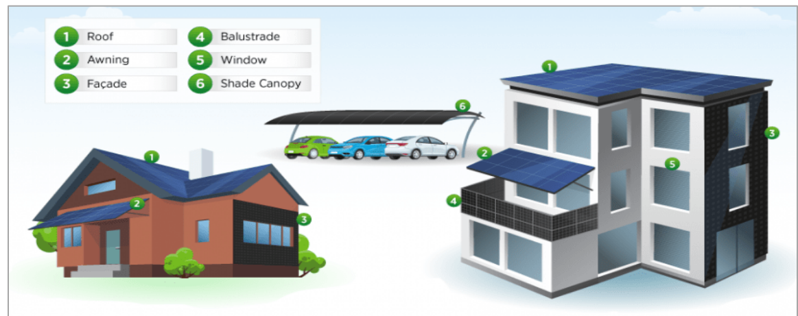
Figure 5.9 Examples of Building-Mounted Solar Systems Source: US Department of Energy
